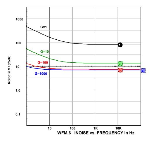
SPICE Waveforms of voltage noise spectral density (RTI)
