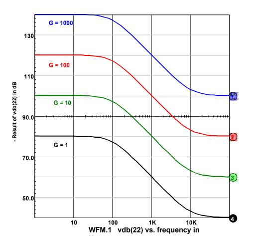
**SPICE** Waveform of common mode rejection
