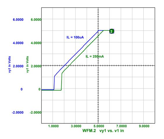
SPICE Waveforms of dropout characteristics
