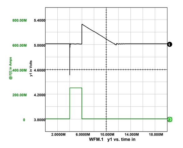
SPICE Waveforms of load transient response
