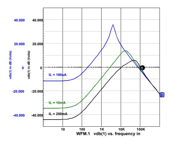
**SPICE** Waveforms of output impedance
