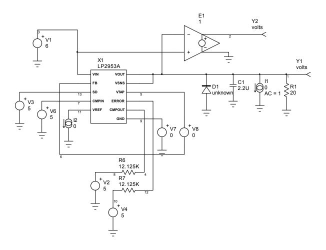
SPICE test circuit for manufacturer's test conditions
