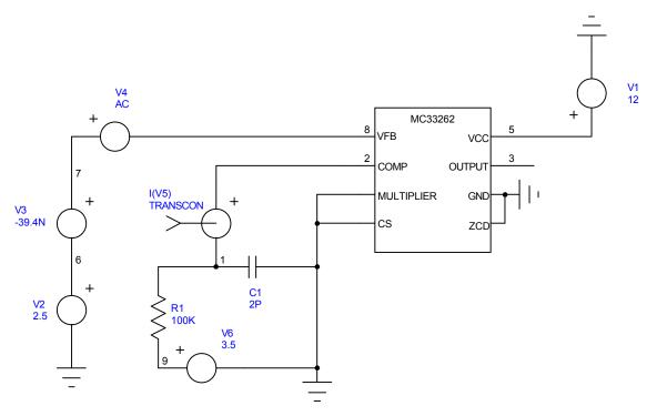
Figure 5.4.1. Error Amp Transconductance and Phase Test Fixture.
