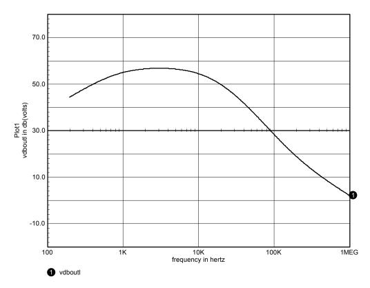
Figure 5.4.2: SPICE waveform of Open-Loop Voltage Gain Vs Frequency
