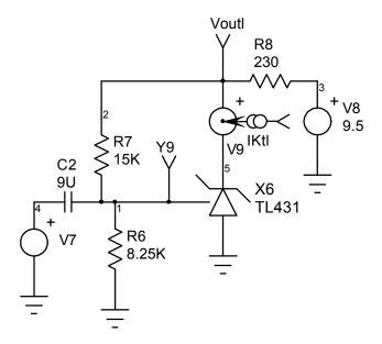
Figure 5.4.1. SPICE test fixture for Open loop Dynamic Gain.
